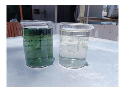
Electrocoagulation Process: In an electrocoagulation system, two electrodes (typically made of aluminum or iron) are immersed in the wastewater or effluent to be treated. When an electric current is applied to the electrodes, it causes several simultaneous electrochemical reactions to occur:
